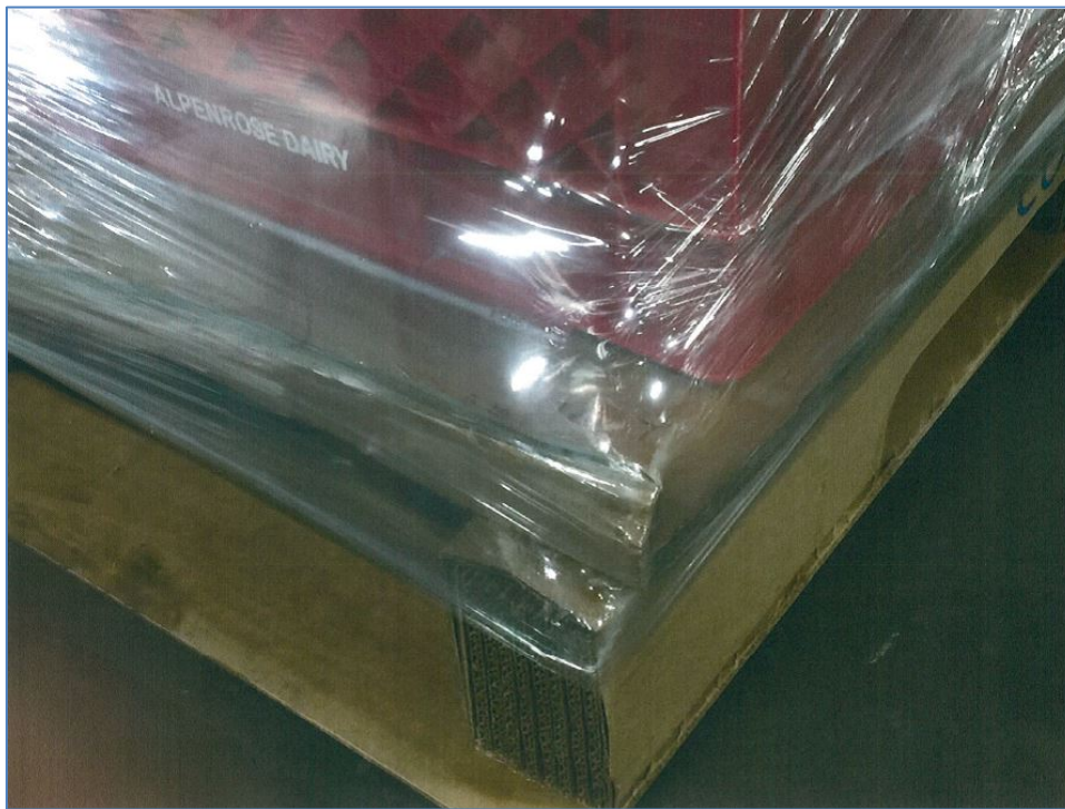
Palletized milk crates that have been shrink wrapped. The corner of the pallet began to rip away from the sides of the pallet when staff attempted to move it to the staging area.
