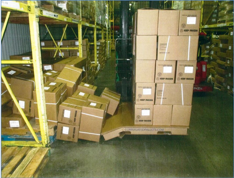
Cardboard pallet loaded with 50 cases of beef patties, each weighing 40 pounds; staff were not able to move the pallet because it crumbled.
