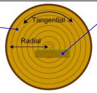
The orientation of the cells across the width and thickness of lumber components are usually a combination of the tangential and radial direction.
